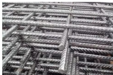
Concrete Reinforcing Mesh
